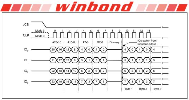
Figure 26b. Word Read Quad I/O Instruction (Previous instruction set M5-4 = 10, SPI Mode only)
