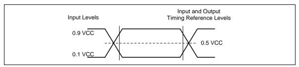
Figure 59. AC Measurement I/O Waveform
