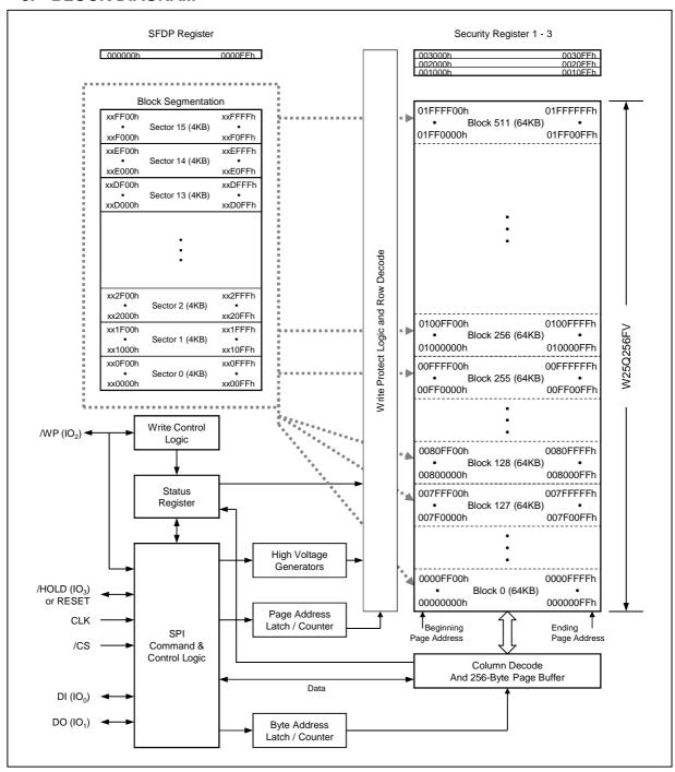
Figure 2. W25Q256FV Serial Flash Memory Block Diagram
