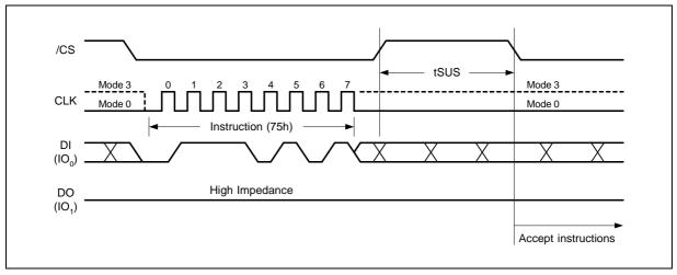
Figure 35a. Erase/Program Suspend Instruction (SPI Mode)
