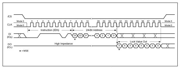
Figure 54a. Read Block Lock Instruction (SPI Mode) 32-Bit Address is required when the device is operating in 4-Byte Address Mode
