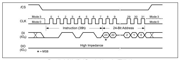
Figure 52a. Individual Block/Sector Lock Instruction (SPI Mode)
