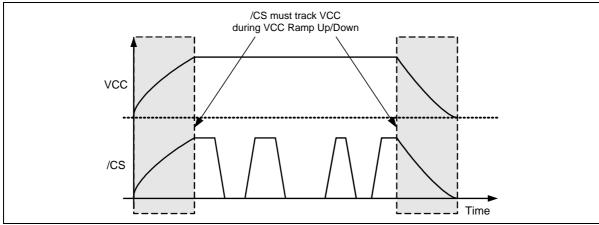
Figure 58b. Power-up, Power-Down Requirement
