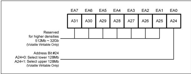
Figure 4e. Extended Address Register
