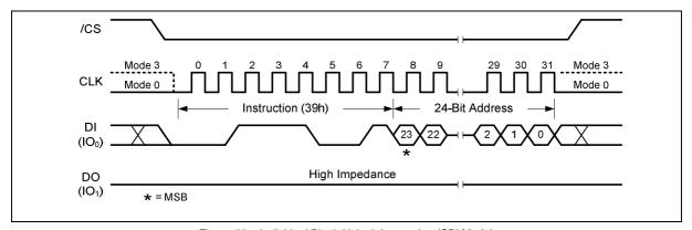
Figure 53a. Individual Block Unlock Instruction (SPI Mode)
