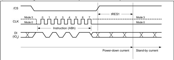
Figure 38a. Release Power-down Instruction (SPI Mode)
