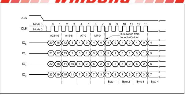
Figure 27b. Octal Word Read Quad I/O Instruction (Previous instruction set M5-4 = 10, SPI Mode only)
