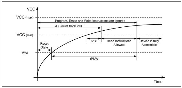
Figure 58. Power-up Timing and Voltage Levels
