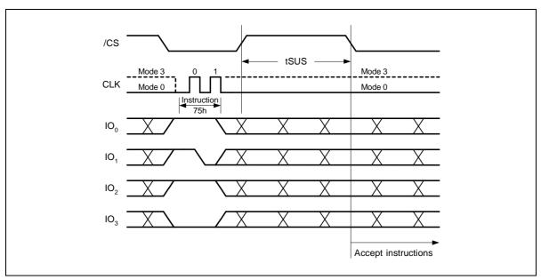
Figure 35b. Erase/Program Suspend Instruction (QPI Mode)
