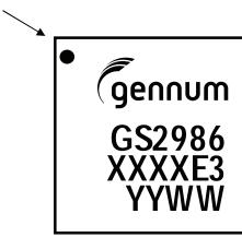
XXXX - Last 4 digits (excluding decimal) of SAP Batch Assembly (FIN) as listed on Packing Slip. E3 - Pb-free & Green indicator YYWW - Date Code
