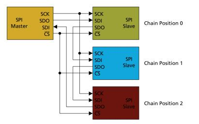
Figure 4-10: Daisy Chained SPI Bus
