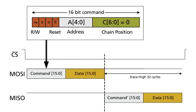
Figure 4-6: Single Device Write
