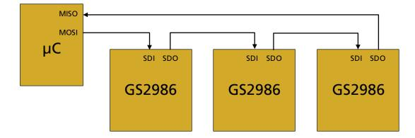
Figure 4-12: Three Devices in Daisy Chain Configuration
