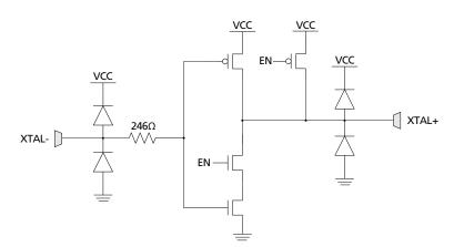
Figure 3-7: High-speed Crystal Oscillator I/O (XTAL-, XTAL+)
