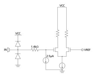
Figure 3-3: Low-speed Input with weak internal pull-down (DDI\_SEL0, DDI\_SEL1)
