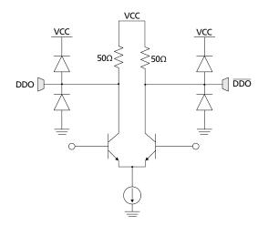
Figure 3-5: High-speed Outputs (DDO1/RCO, DDO1/RCO, DDO0)
