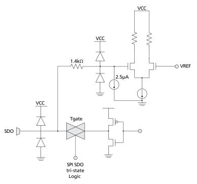
Figure 3-9: SPI Output/EQ Control (SDO/EQ1\_EN)
