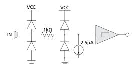
Figure 3-8: SPI Inputs/EQ Ctrl (CS/EQ3\_EN, SCK/EQ2\_EN, SDI/EQ0\_EN)
