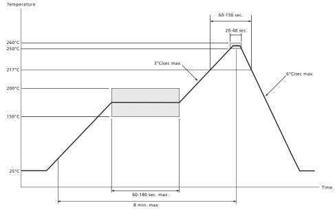
Figure 6-1: Maximum Pb-free Solder Reflow Profile
