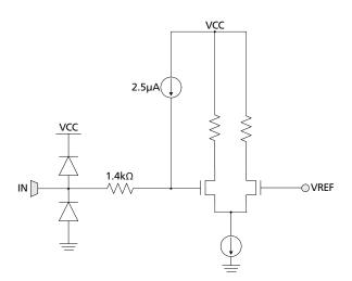
Figure 3-2: Low-speed Input with weak internal pull-up (HIF, DDO1\_DISABLE)
