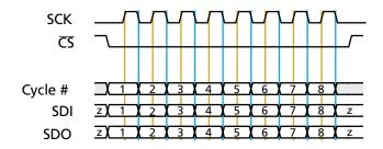
Figure 4-4: Data Clock Alignment
