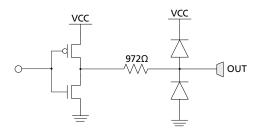
Figure 3-4: Low-speed Outputs (LOCKED, LOS, SD/HD)
