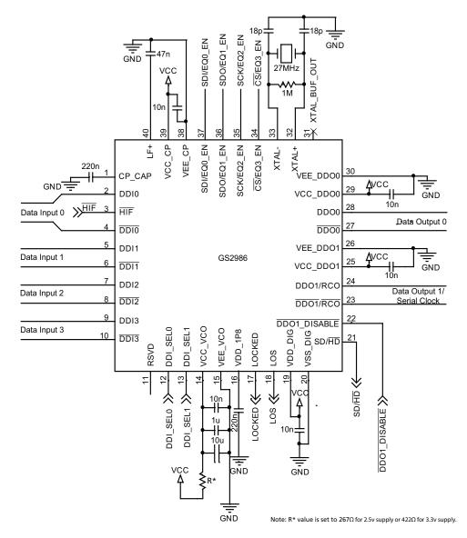
Figure 5-1: GS2986 Typical Application Circuit
