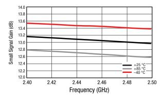
Figure 4. Small Signal Gain (IS21I) vs Frequency and Temperature, Narrow Band
