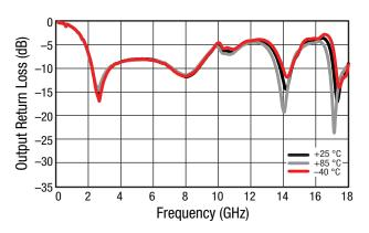
Figure 24. Small Signal Output Return Loss (| S22 |) vs Frequency and Temperature, Wide Band
