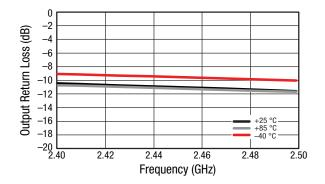
Figure 7. Small Signal Output Return Loss (IS22I) vs Frequency and Temperature, Narrow Band
