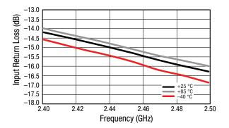
Figure 5. Small Signal Input Return Loss (IS11) vs Frequency and Temperature, Narrow Band
