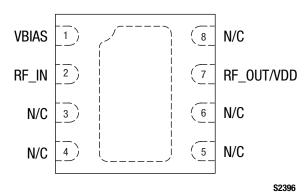
Figure 2. SKY67014-396LF Pinout – 8-Pin DFN (Top View)
