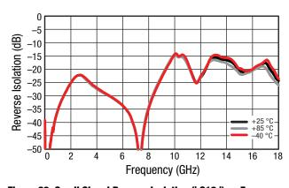
Figure 23. Small Signal Reverse Isolation (| S12 |) vs Frequency and Temperature, Wide Band
