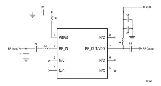
Figure 28. SKY67014-396LF Evaluation Board Schematic
