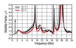
Figure 12. Stability Factor  $(\mu 1)$  vs Frequency and Temperature, Wide Band
