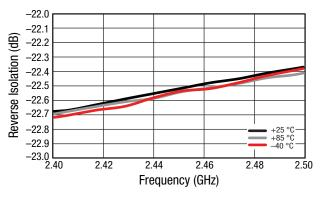
Figure 19. Small Signal Reverse Isolation (IS12I) vs Frequency and Temperature, Narrow Band
