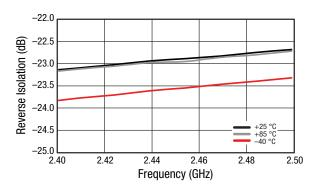
Figure 6. Small Signal Reverse Isolation (IS12I) vs Frequency and Temperature, Narrow Band
