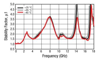
Figure 25. Stability Factor ( $\mu$ 1) vs Frequency and Temperature, **Wide Band**
