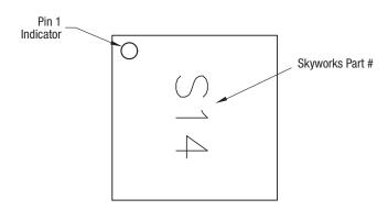
Figure 30. Typical Case Markings (Top View)
