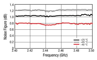
Figure 16. Noise Figure vs Frequency and Temperature, Narrow Band (Includes EVB Insertion Losses)
