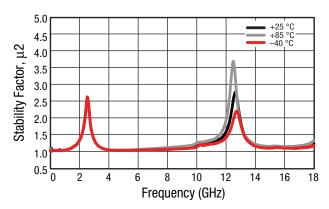
Figure 26. Stability Factor (µ2) vs Frequency and Temperature, Wide Band
