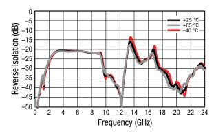
Figure 10. Small Signal Reverse Isolation (I S12 I) vs Frequency and Temperature, Wide Band
