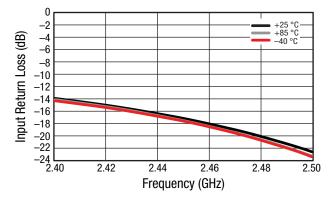
Figure 18. Small Signal Input Return Loss (IS11I) vs Frequency and Temperature, Narrow Band
