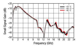
Figure 8. Small Signal Gain (IS21I) vs Frequency and Temperature, Wide Band
