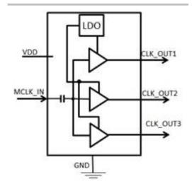
Figure 1. Simplified Block Diagram
