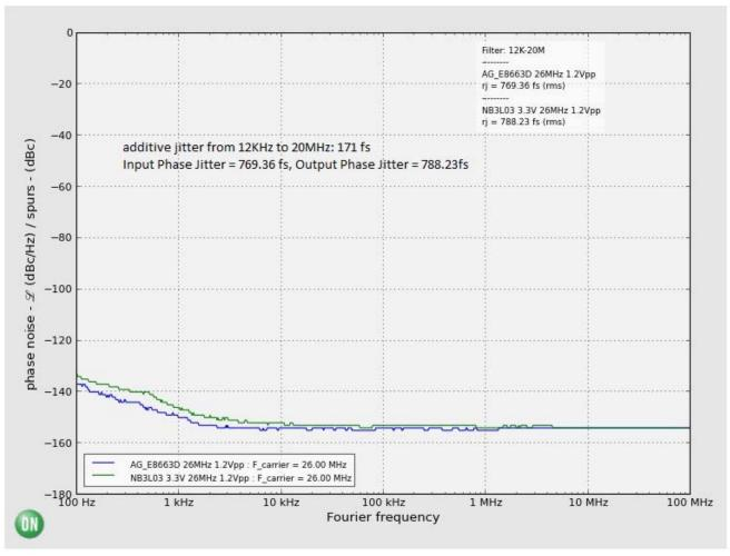
Figure 2. Typical Phase Jitter @ 26 MHz, INT Range (12 kHz to 20 MHz)
