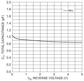
Figure 6 Typical Total Capacitance vs. Reverse Voltage
