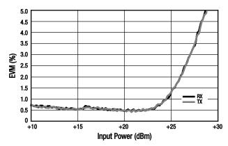
Figure 6. EVM vs Input Power (@ 2.45 GHz, 54 bps)
