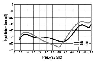
**Figure 4. Input Return Loss vs Frequency**
