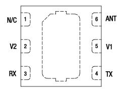
Figure 2. SKY13446-374LF Pinout – 6-Pin MLPD (Top View)
