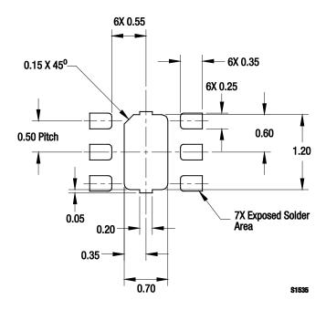
Figure 10. SKY13446-374LF PCB Layout Footprint (Top View)
