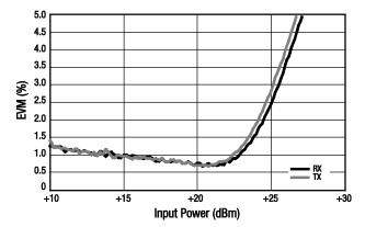
Figure 7. EVM vs Input Power (@ 5.5 GHz, 54 bps)
