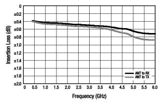
**Figure 3. Insertion Loss vs Frequency**
