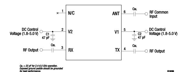
Figure 8. SKY13446-374LF Evaluation Board Schematic
