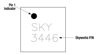
Figure 11. Typical Part Markings (Top View)
