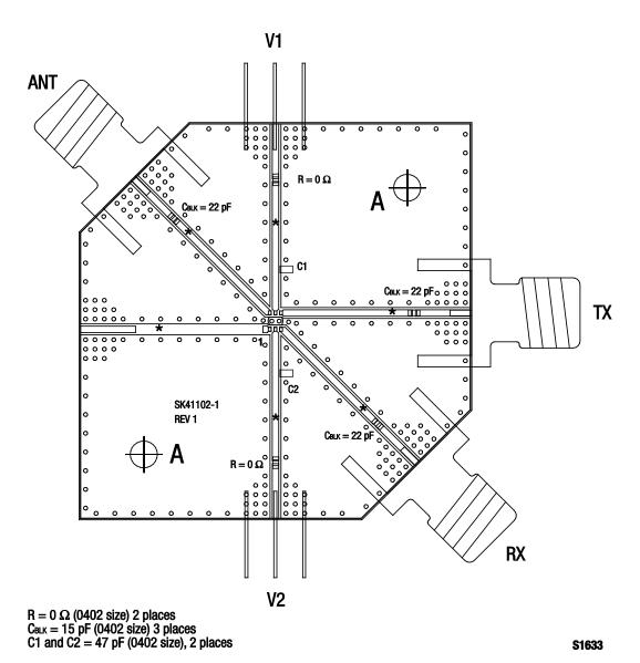
Figure 9. SKY13446-374LF Evaluation Board Assembly Diagram
