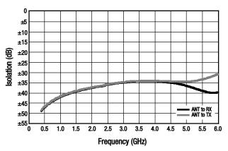
Figure 5. Isolation vs Frequency
