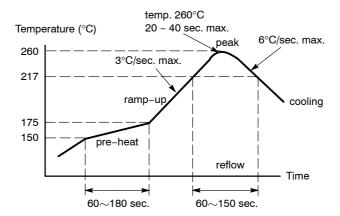
Figure 4. Recommended Reflow Soldering Profile
