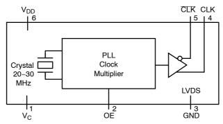
Figure 1. Simplified Logic Diagram
