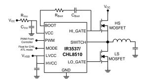
Figure 1: Basic Applications Circuit
