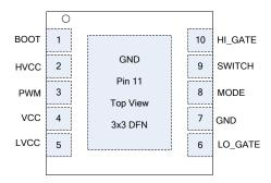
Figure 2: IR3537/CHL8510 Package Top View
