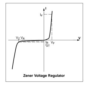
**ELECTRICAL CHARACTERISTICS** ( $T_L = 30^{\circ}C$  unless otherwise noted,  $V_F = 1.5$  V Max @  $I_F = 200$  mAdc for all types)
