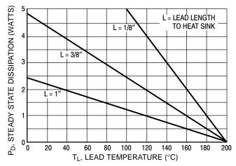
Figure 1. Power Temperature Derating Curve
