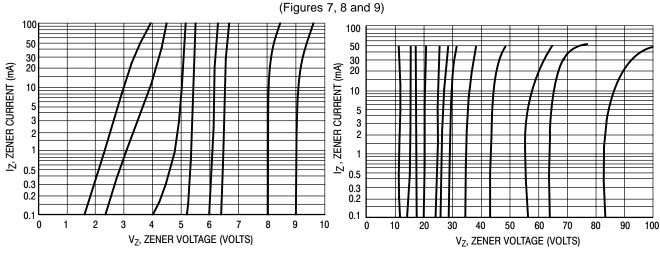
Figure 7.  $V_Z = 3.3$  thru 10 Volts
