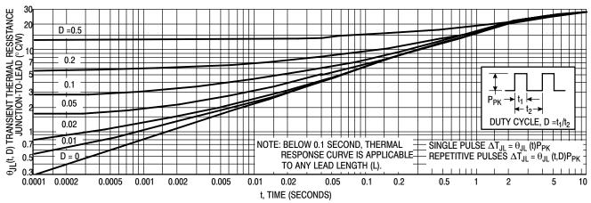
Figure 2. Typical Thermal Response L, Lead Length = 3/8 Inch
