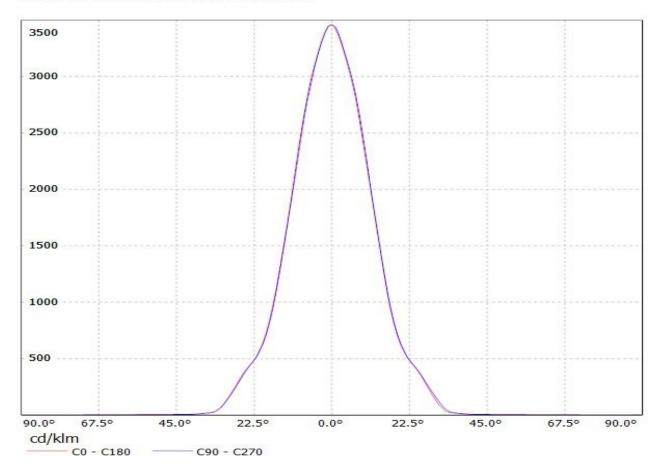
Luminaire: LEDiL Oy CN13105\_LENA-M\_(Soleriq\_E30) Eff.85% Lamps: 1 x Osram Soleriq E30 (1240lm@250mA)
