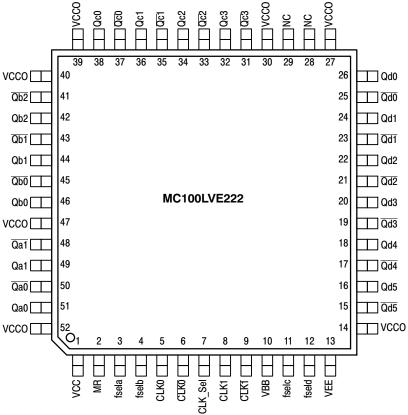
Figure 1. Pinout Assignment (Top View)
