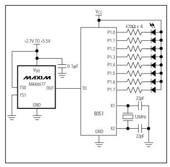
Figure 5. Interfacing with a  $\mu$ C
