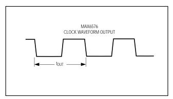
Figure 1. MAX6576 Timing Diagram
