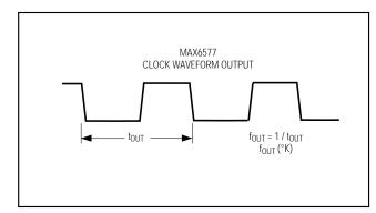
Figure 2. MAX6577 Timing Diagram
