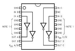
Note 1: Pins 4-7 and 14-17 are electrically connected
