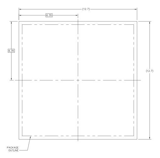
PCB DESIGN GUIDELINES - SOLDER MASK OPENING PATTERN 1
