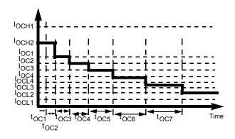
Figure 15. Over-current Profile with OCHI bit set to '1'
