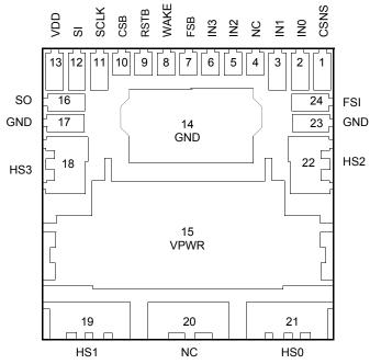
Figure 3. 09XS3400 Pin Connections
