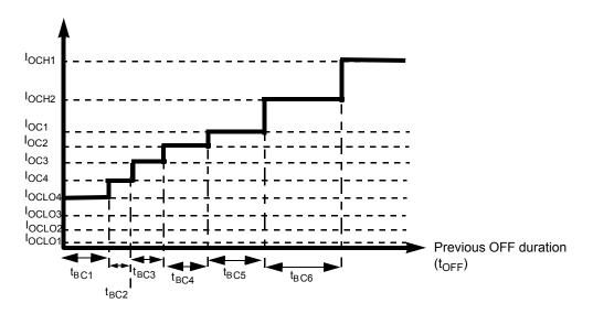
Figure 6. Bulb Cooling Management
