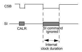
If the negative CSB pulse is outside a predefined time range (from  $t_{\text{CSB}(\text{MIN})}$  to  $t_{\text{CSB}(\text{MAX})}$ ), the calibration event will be ignored and the internal clock will be unaltered or reset to its default value ( $f_{\text{PWM}(0)}$ ) if this was not calibrated before.
