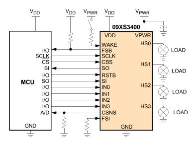
Figure 1. 09XS3400 Simplified Application Diagram
