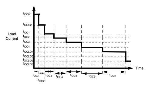
Figure 5. Over-current Shutdown Protection
