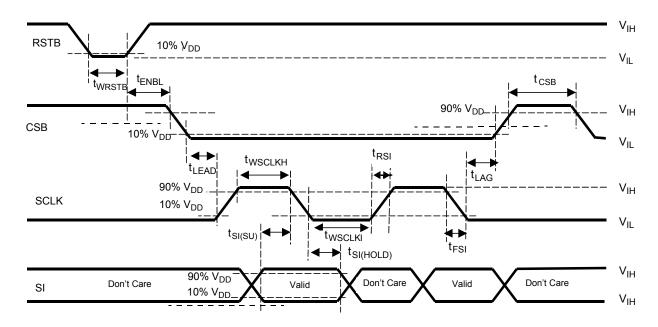
Figure 7. Input Timing Switching Characteristics
