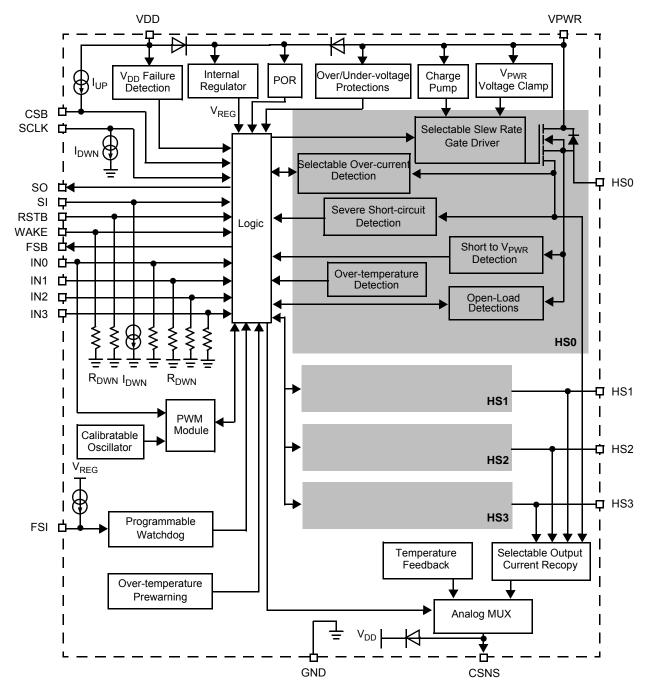
Figure 2. 09XS3400 Simplified Internal Block Diagram
