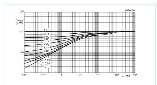
Fig 1. Thermal resistance from junction to tie-point as a function of pulse duration; lead length 4 mm
