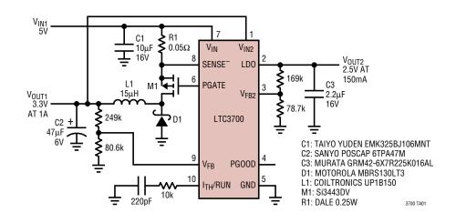
5V Input Supply to 3.3V/1A High Efficiency Output and 2.5V/150mA Low Noise Output
