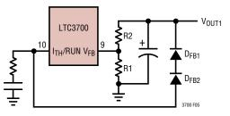
Figure 5. Foldback Current Limiting
