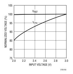
Figure 3. Line Regulation of  $V_{\text{REF}}$  and  $V_{\text{ITH}}$
