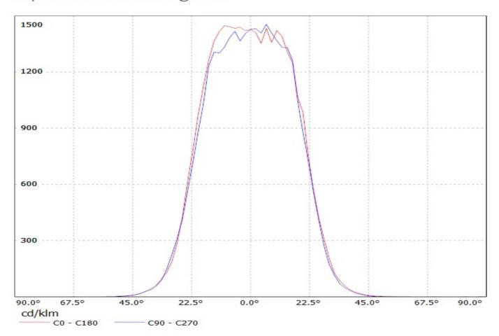
Luminaire: LEDiL Oy CN13158\_LENA-WAS\_(CL-L340) Eff.83.7% Lamps: 1 x CL-L340 (929.39Im@250mA)
