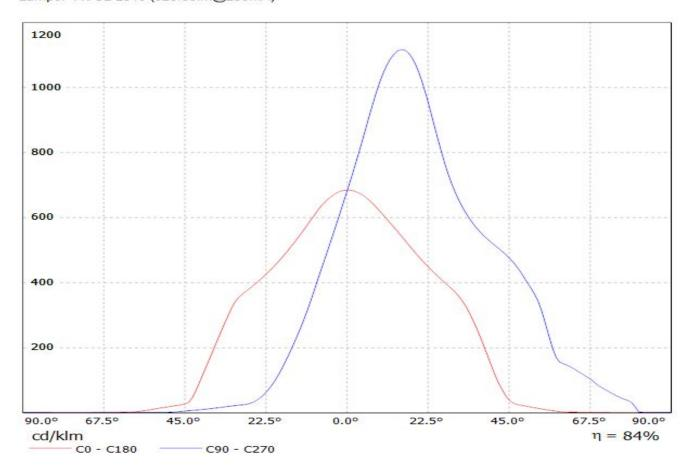
Luminaire: LEDiL Oy CN13168\_LENA-WAS-DL\_(CL-L340) Eff.79.2% Lamps: 1 x CL-L340 (929.39Im@250mA)
