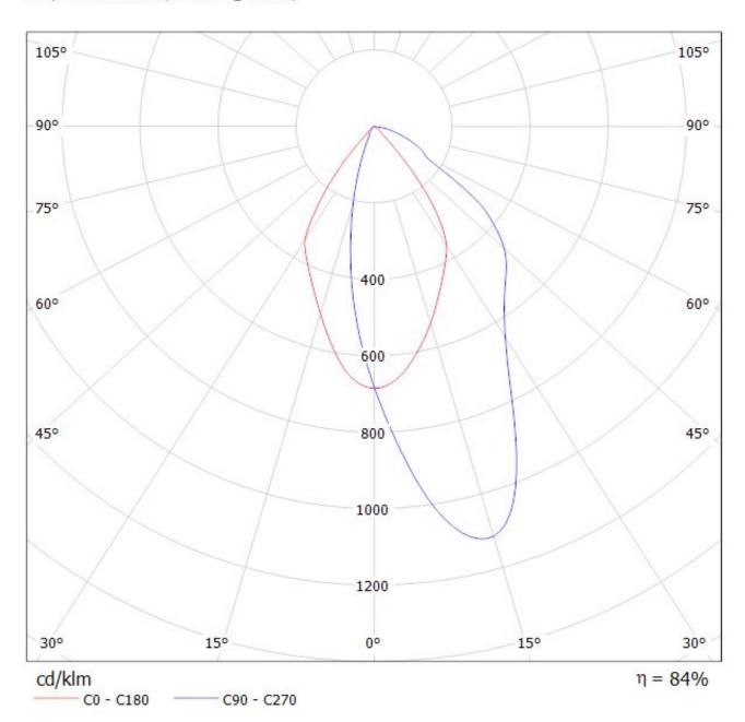
Luminaire: LEDiL Oy CN13168\_LENA-WAS-DL\_(CL-L340) Eff.79.2% Lamps: 1 x CL-L340 (929.39Im@250mA)
