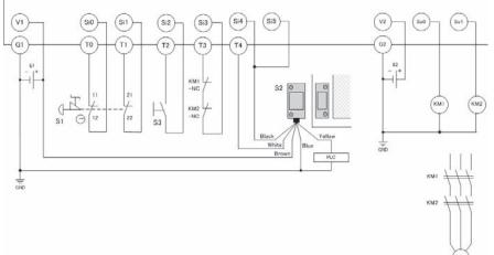
E1 and E2:24-VDC power suppliesS1:Emergency stop pushbuttonS2:D40A Non-contact SwitchS3:Reset switchKM1and KM2:ContactorsM:Motor
