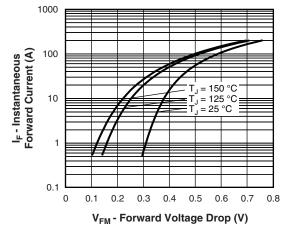
Fig. 1 - Maximum Forward Voltage Drop Characteristics (Per Leg)
