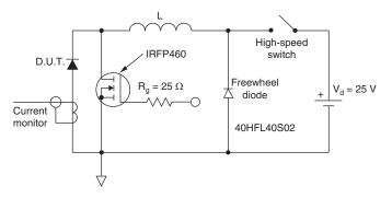
Fig. 8 - Unclamped Inductive Test Circuit
