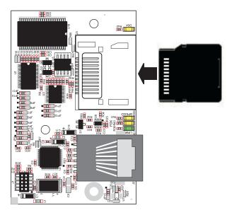
Figure 14. Insertion/Removal of microSD Card
