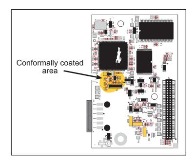
Figure A-6. RCM4300 Areas Receiving Conformal Coating
