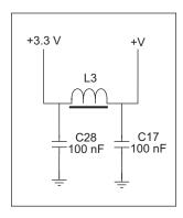
Figure 13. Analog Supply Circuit
