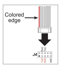
• SIMPLE3WIRE.C—This program demonstrates basic RS-232 serial communication. Lower case characters are sent on TxC, and are received by RxD. The received characters are converted to upper case and are sent out on TxD, are received on RxC, and are displayed in the Dynamic C STDIO window.
