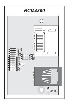
Figure A-5. Location of RCM4300 Configurable Positions
