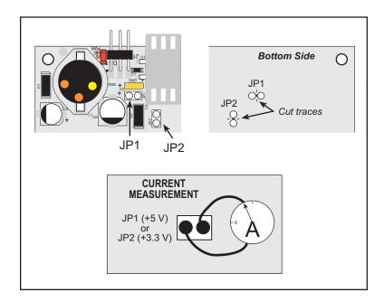
Figure B-5. Prototyping Board Current-Measurement Option
