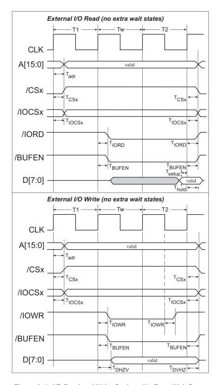
Figure A-4. I/O Read and Write Cycles—No Extra Wait States
