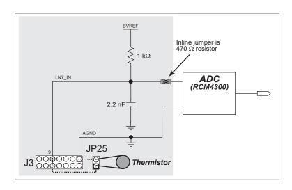
Figure B-7. Prototyping Board Thermistor Input
