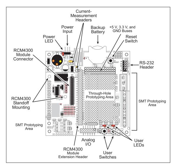
Figure B-1. Prototyping Board
