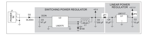
Figure B-3. Prototyping Board Power Supply
