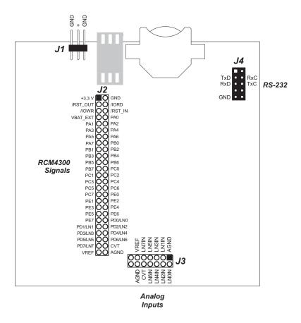
Figure B-4. Prototyping Board Pinout
