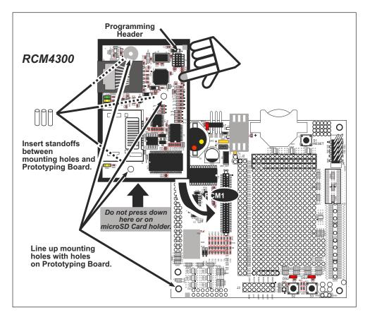
Figure 3. Install the Module on the Prototyping Board
