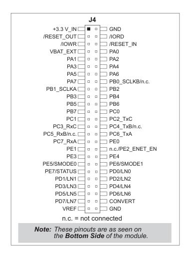
Figure 6. RCM4300 Pinout
