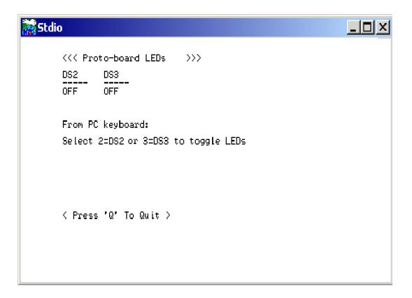
Press "2" or "3" on your keyboard to select LED DS2 or DS3 on the Prototyping Board. Then follow the prompt in the Dynamic C **STDIO** window to turn the LED ON or OFF. A logic low will light up the LED you selected.
