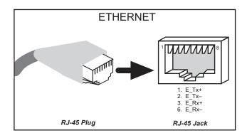
Figure 8. RJ-45 Ethernet Port Pinout
