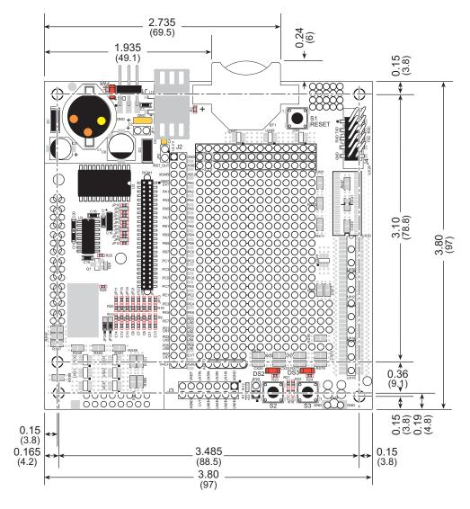
Figure B-2. Prototyping Board Dimensions
