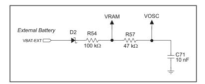
Figure C-2. RCM4300 Backup Battery Circuit
