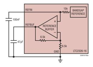
Figure 5a. LTC2326-16 Internal Reference Circuit
