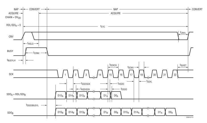
Figure 12. Chain Mode Timing Diagram
