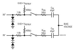
Figure 3. The Equivalent Circuit for the Differential Analog Input of the LTC2326-16
