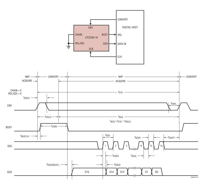
Figure 10. Using a Single LTC2326-16 in Normal Mode
