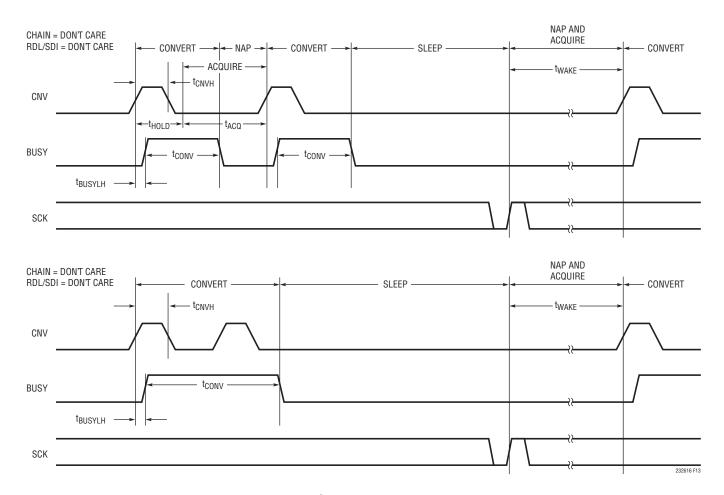
Figure 13. Sleep Mode Timing Diagram
