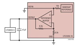
Figure 5c. Overdriving REFBUF Using the LTC6655-5
