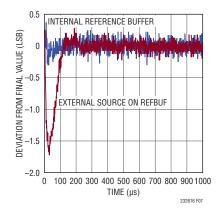
Figure 7. Transient Response of the LTC2326-16
