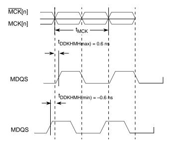
Figure 5. Timing Diagram for  $t_{\mbox{\scriptsize DDKHMH}}$
