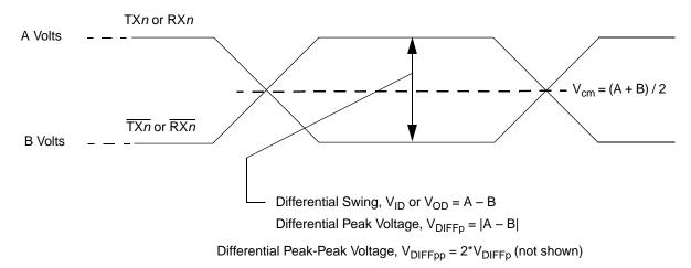
Figure 15. Differential Voltage Definitions for Transmitter or Receiver
