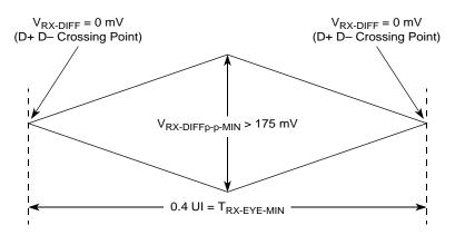
Figure 28. Minimum Receiver Eye Timing and Voltage Compliance Specification
