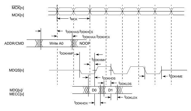
Figure 6. DDR2 SDRAM Output Timing Diagram
