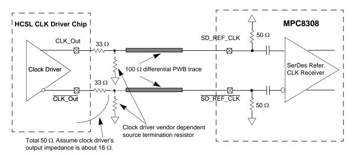
Figure 20. DC-Coupled Differential Connection with HCSL Clock Driver (Reference Only)
