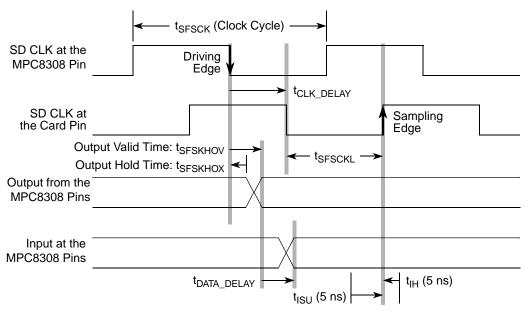
Figure 35. Full Speed Output Path
