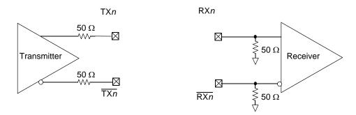
Figure 26. SerDes Transmitter and Receiver Reference Circuits
