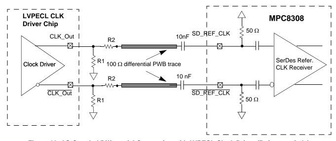
Figure 22. AC-Coupled Differential Connection with LVPECL Clock Driver (Reference Only)
