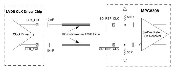
Figure 21. AC-Coupled Differential Connection with LVDS Clock Driver (Reference Only)
