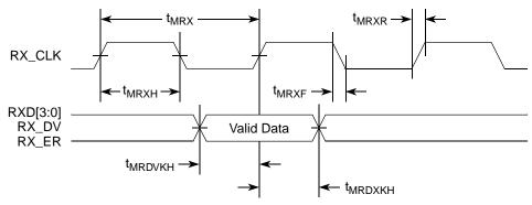
Figure 9. MII Receive AC Timing Diagram RMII AC Timing Specifications
