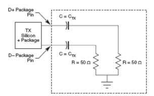
Figure 29. Compliance Test/Measurement Load
