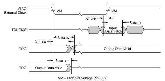
Figure 44. Test Access Port Timing Diagram
