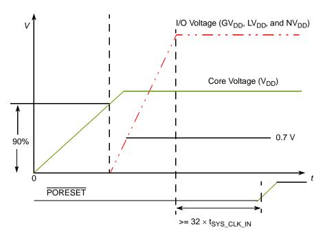
Figure 3. Power-Up Sequencing Example
