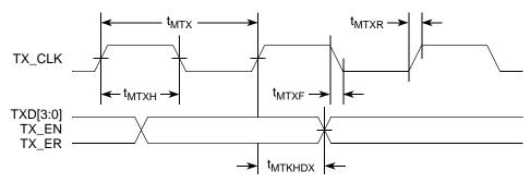
Figure 8. MII Transmit AC Timing Diagram
