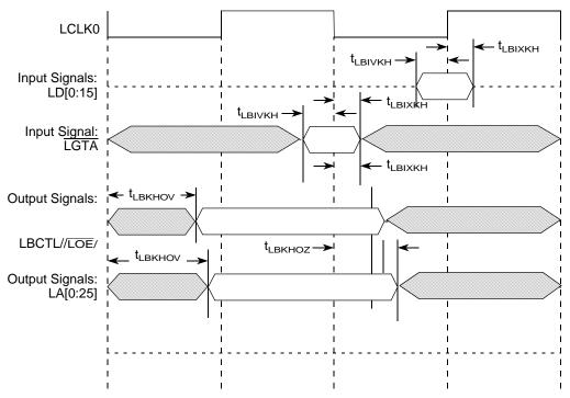
Figure 31. Local Bus Signals, Non-Special Signals Only
