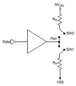
Figure 55. Driver Impedance Measurement
