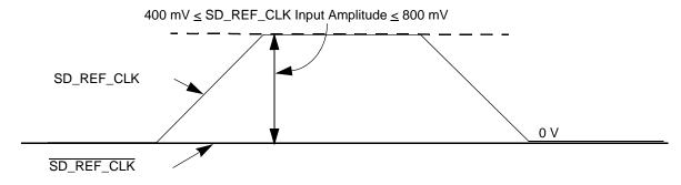
Figure 19. Single-Ended Reference Clock Input DC Requirements
