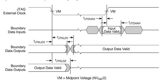
Figure 43. Boundary-Scan Timing Diagram
