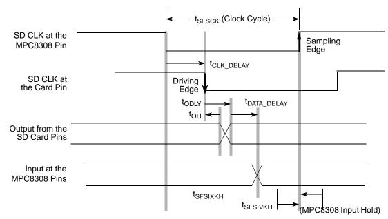
Figure 36. Full Speed Input Path
