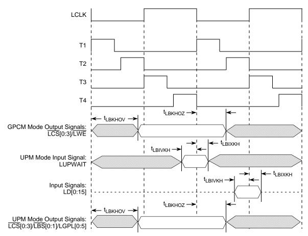
Figure 33. Local Bus Signals, GPCM/UPM Signals for LCCR[CLKDIV] = 4
