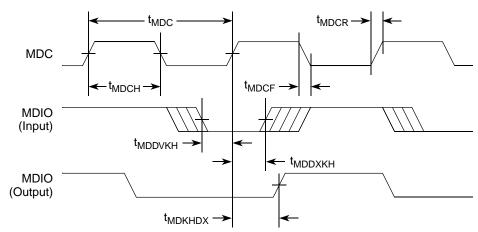
Figure 12. MII Management Interface Timing Diagram
