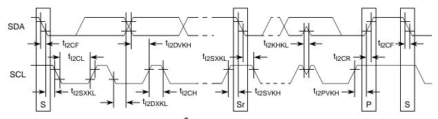
Figure 46. I<sup>2</sup>C Bus AC Timing Diagram
