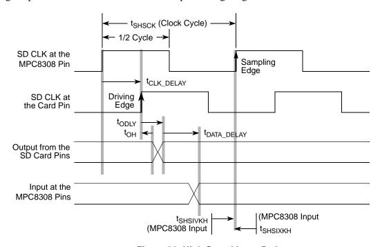
Figure 39. High Speed Input Path
