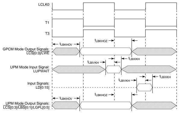
Figure 32. Local Bus Signals, GPCM/UPM Signals for LCCR[CLKDIV] = 2
