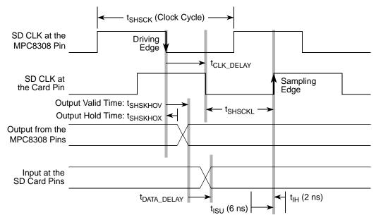
Figure 38. High Speed Output Path
