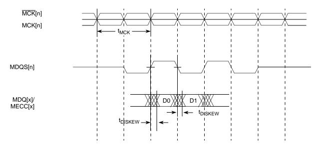
Figure 4. Timing Diagram for t<sub>DISKEW</sub>
