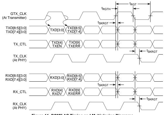
Figure 11. RGMII AC Timing and Multiplexing Diagrams
